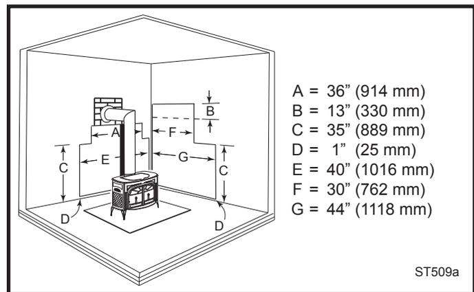
**Fig. 25** Parallel installation with rear wall pass-through, with stove, connector and wall shields. Wall shields may meet at corner. Connector heat shield extends 28" (710mm) above flue collar, or below elbow, whichever is less. Wall pass-through must comply with codes.
